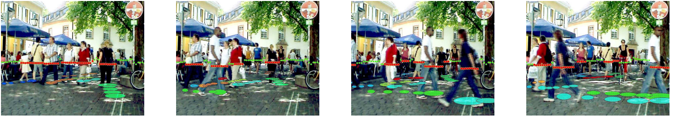
Fig. 7. Four images of the outdoor experiments carried out in the inner city of Freiburg. The information of the laser range finder and the tracking system were projected onto a recorded video sequence. The images from left to right show the tracking results at timesteps t = 335, 353, 365 and 381 . Laser range measurements are shown as small green dots (background) or small red dots (detected pedestrians). The traces of the observed pedestrians are drawn with colored ellipses.
