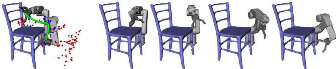
Fig. 7. Our approach can clasp loops that are not directly reachable from the robot's initial configuration. Here, the RRT spans from the initial configuration to the free space in front of the chair, visualized by the grasp center point in red. The solution's 30 nodes are shown in blue and the optimized solution is shown in green. The search terminated after 606 cycles and with 248 nodes in the tree.
