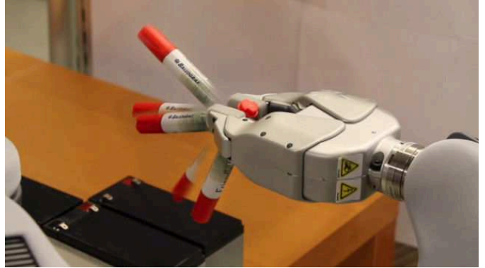
Fig. 1. In-hand manipulation using resources extrinsic to the robot requires representations that describe the hand-object dynamical system including the task-relevant parts of the environment. Here, the robotic gripper was placed in different positions and moved down to push the marker-pen against an edge.
